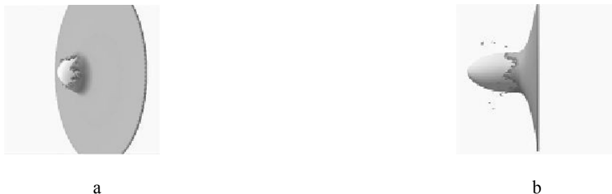
Figure 7. Petals formation in copper plate (projectile velocity – 300 m/s):a - t = 200 \mu s ; b- t = 400 \mu s .
