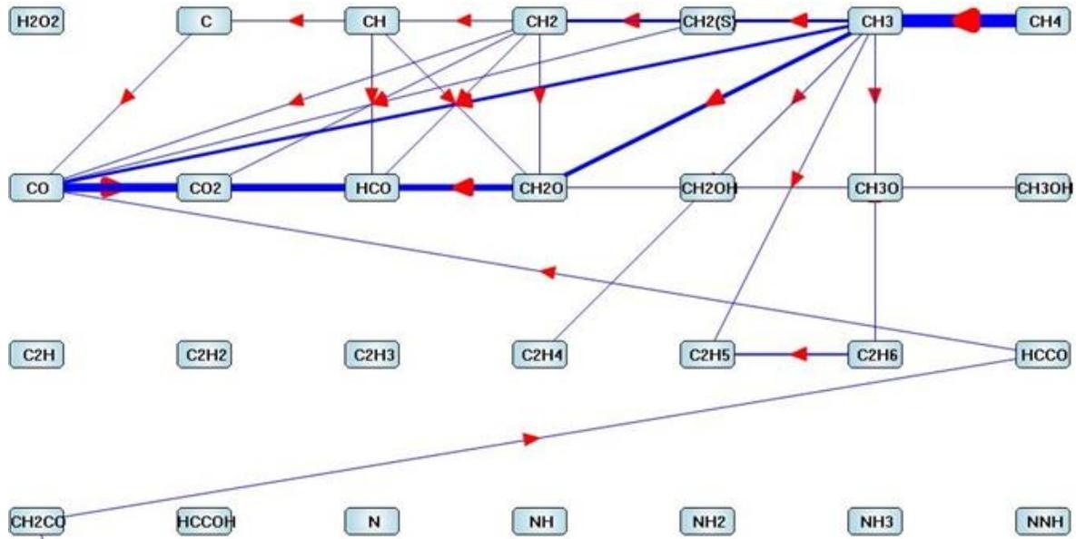
Figure 8: Elemental flux analysis for carbon atoms in a non-preheated stoichiometric premixed methane-air flame
