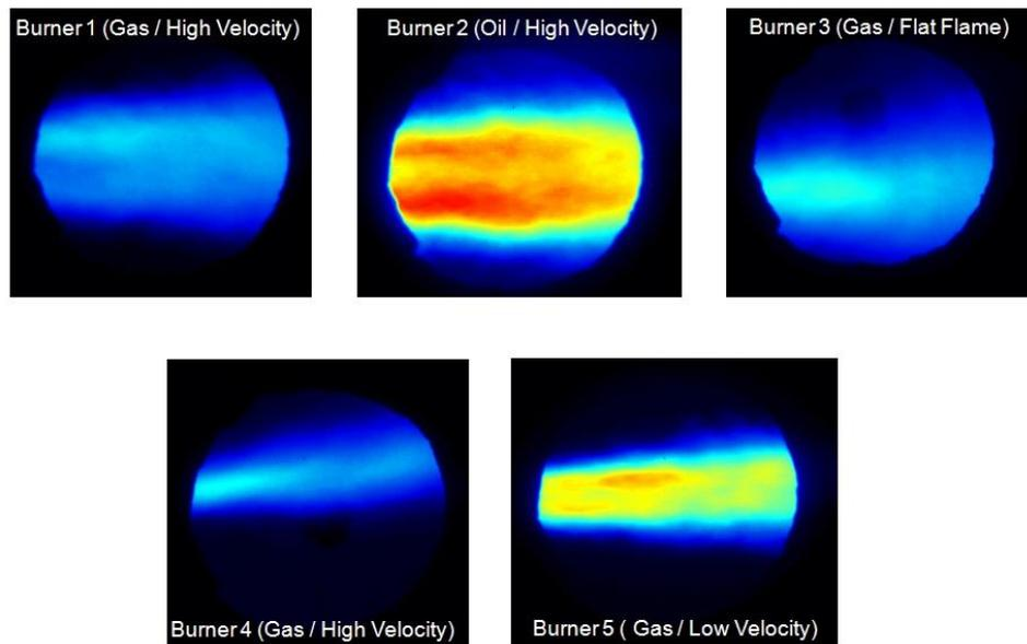
Figure 2: OH chemoluminescence images of the investigated burners
