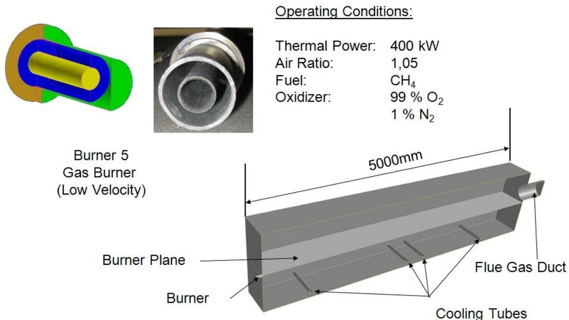
**Figure 5: Geometry and boundary conditions**
