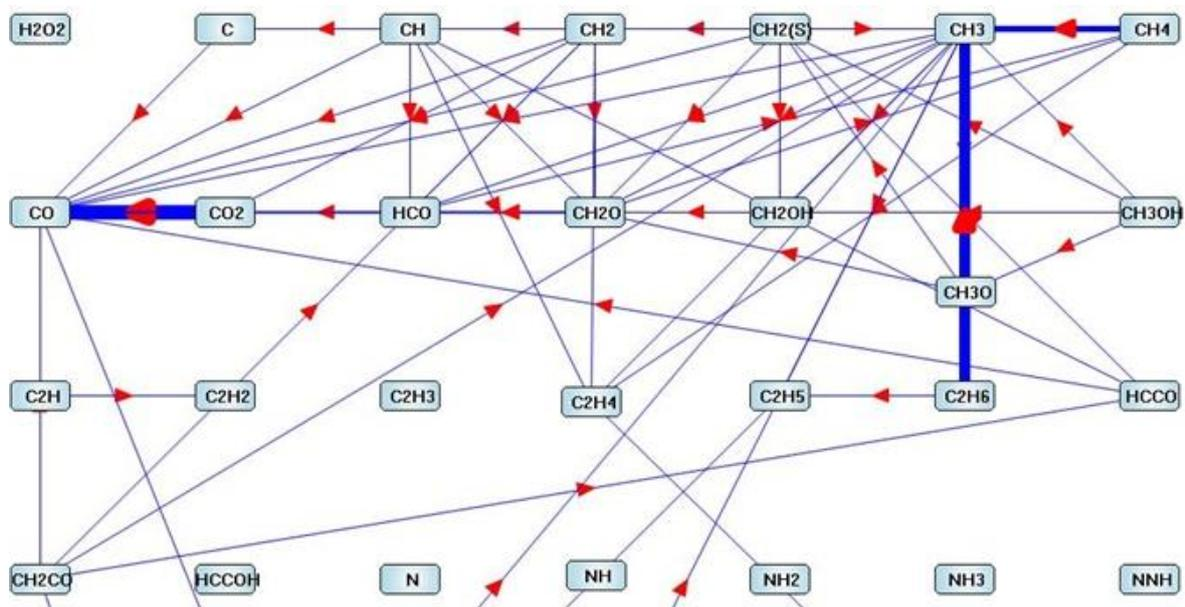
Figure 9: Elemental flux analysis for carbon atoms in a non-preheated stoichiometric premixed methane-oxygen flame
