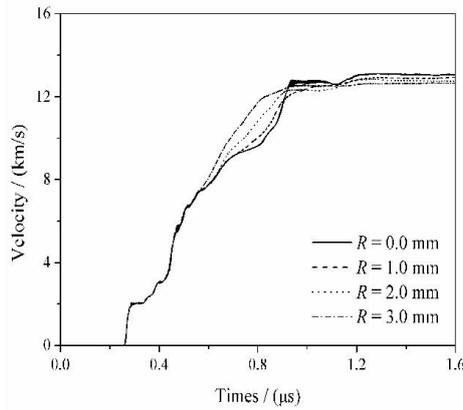
**Figure 3:** Velocity histories of the flier plate at different radial positions in the initial model.
