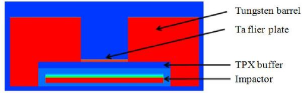
**Figure 2:** Schematic of the initial model
