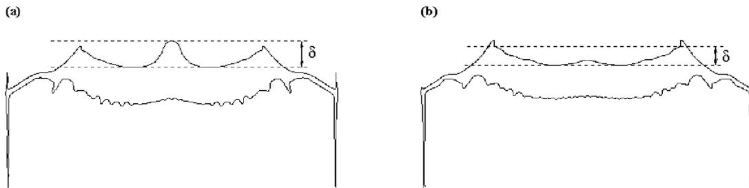
Figure 1: Definitions of planarity parameters  $\delta$ .
