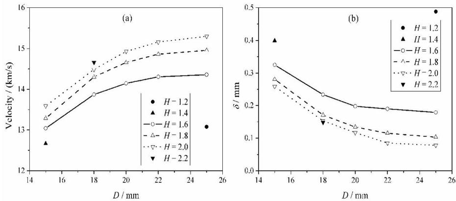
**Figure 7:** The velocity and planarity of the flier plate as a function of the diameter and thickness of the tungsten at  $1.4 \mu\text{s}$ . The black solid dot denotes the result of initial Model.
