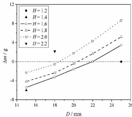
**Figure 6:** The mass difference of the impactor as a function of the diameter and thickness of the tungsten. The horizontal dashed line represents the zero contours of the mass difference.
