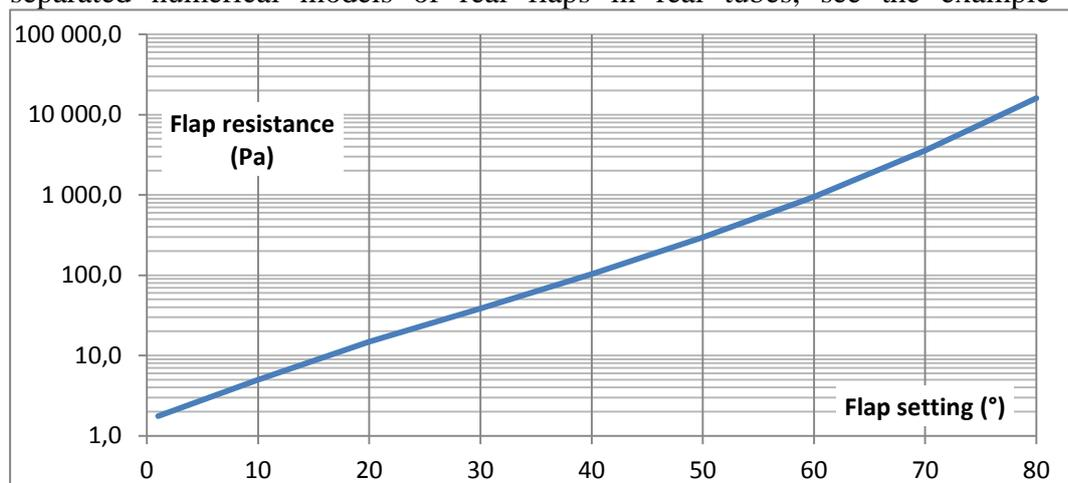
Figure 10: Flap resistance at various setting
