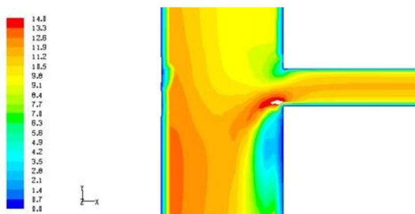
Figure 5: Detail of the velocity field in the connection of the branch 6
