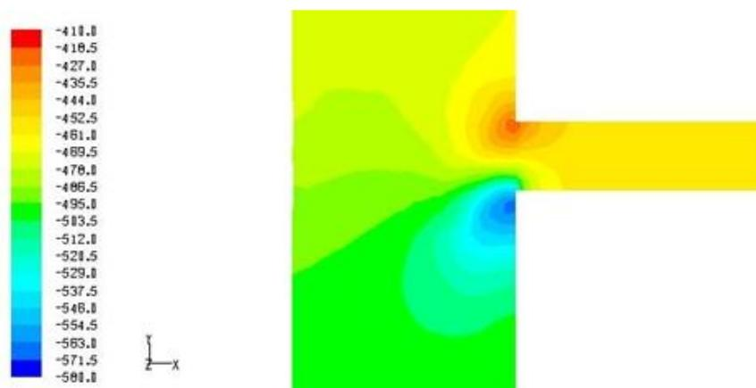
Figure 4: Detail of the pressure field in the connection of the branch 6
