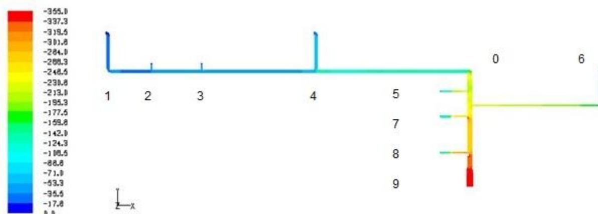
**Figure 3:** Pressure field in solved tube system with connections marking
