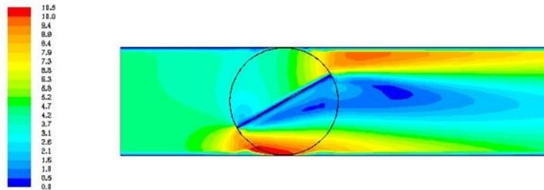
**Figure 14:** Velocity field around the flap in tube at flap setting of 30°
