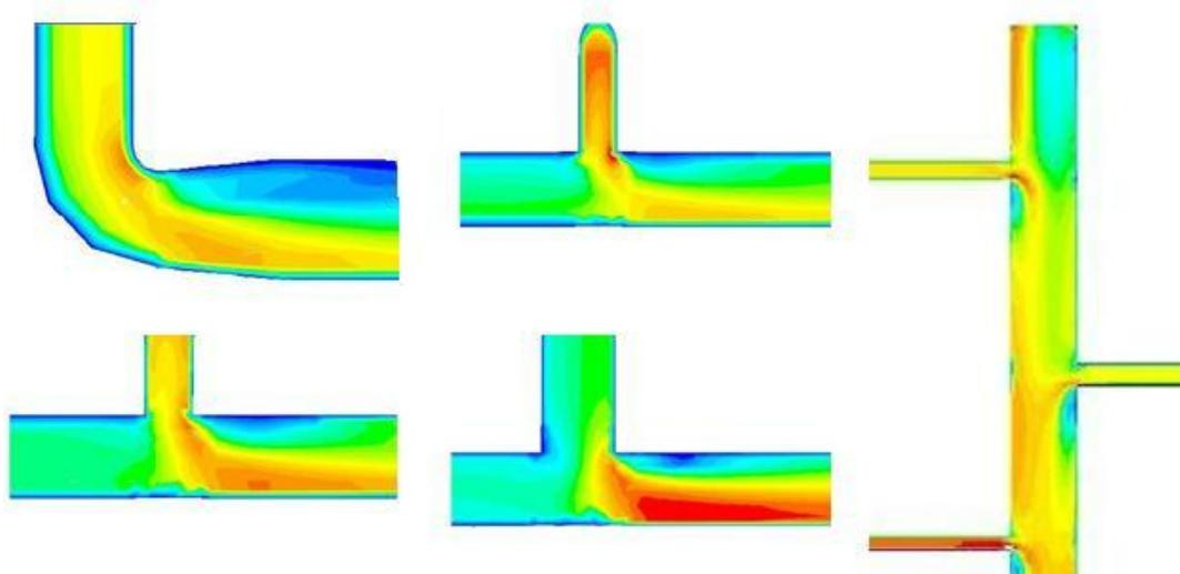
**Figure 17:** Velocity axial profiles at areas of connections No. 1 - 2 (up), 3 - 4 (down), 5 - 6 - 7 (vertical)
