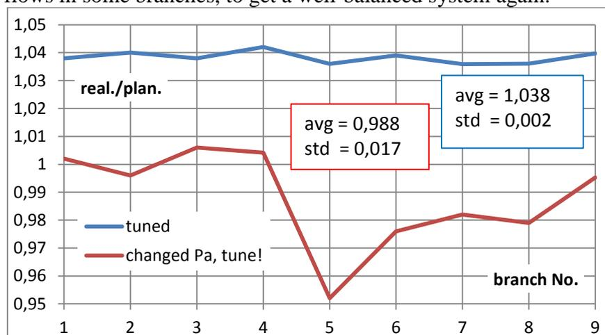
Figure 7: Relative flows in branches 1 to 9 - tuned and unbalanced again by another pressure gradient
