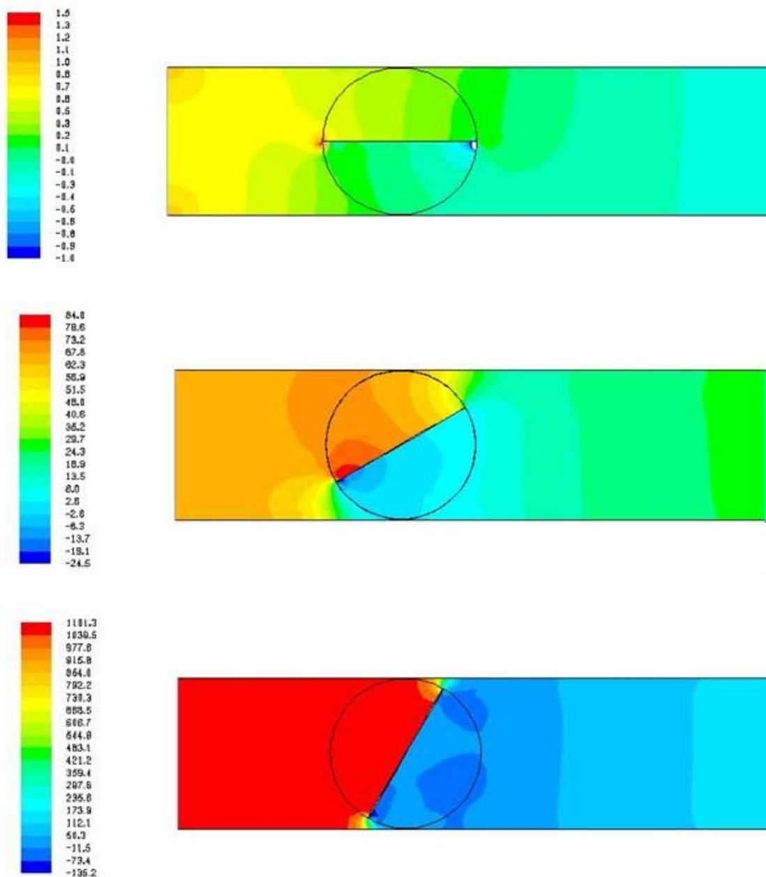
**Figure 11 to 13:** Pressure fields around the flap in tube at flap setting  $0^\circ$  -  $30^\circ$  -  $60^\circ$
