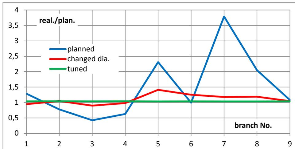
Figure 6: Relative flows in branches 1 to 9 - planned, changed diameters, tuned
