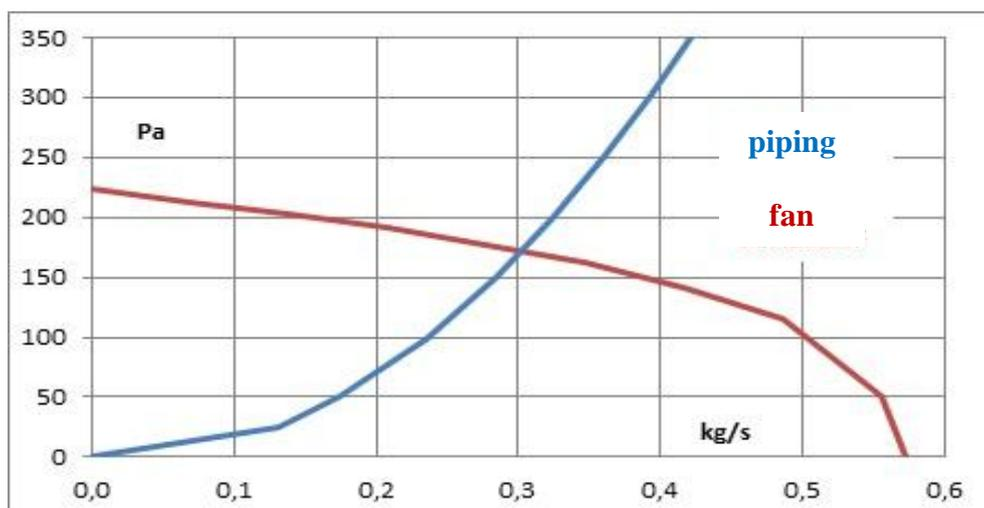
Figure 9: Typical operational point of the system fan + tubing
