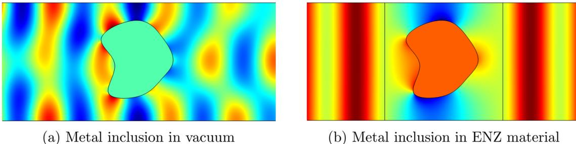
Figure 2: Light incident on an arbitrarily-shaped metal object produces a large degree of scattering (left). When the same object is submerged in a matched ENZ material, the incoming light waves are transmitted and remain planar; the object is invisible (right).
