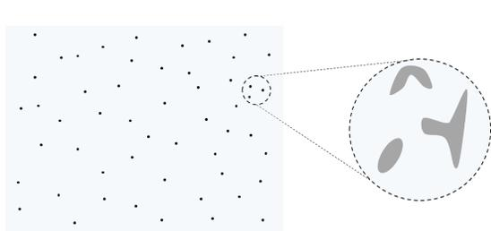
(a) Composite comprised of small particles embedded in a host matrix
