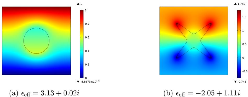
Figure 1: Small silver particles in a dielectric background, illuminated with light at 500 THz. The local electric potential field, as well as the effective permittivity  $\epsilon_{\text{eff}}$  of the composite, is greatly influenced by particle shape.
