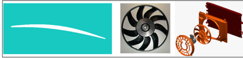
Figure 1: The automotive cooling module, its 9-blades fan and the airfoil of the blade
