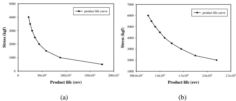
**Figure 8:** Product life curve of bearing for (a) wear depth of 0.5mm and (b) spalling of 6mm<sup>2</sup>
