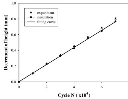
Figure 6: Comparison between test result and computation result for bearing wear test
