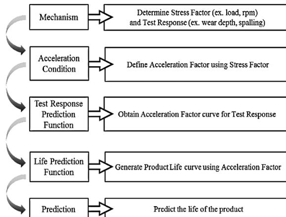
Figure 5: Procedure of accelerated life test coupled with numerical analysis
