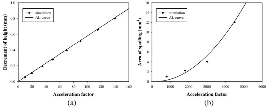
**Figure 7:** Computation by AF and AL-curve of bearing for (a) wear depth and (b) spalling
