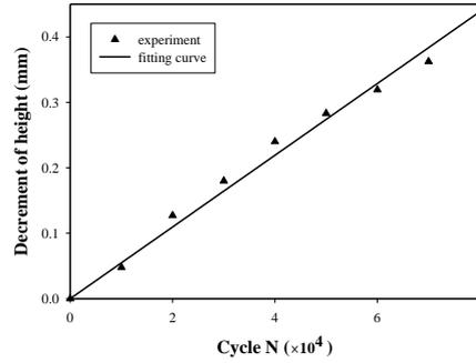
**Figure 3:** Experiment result of wear test for bearing
