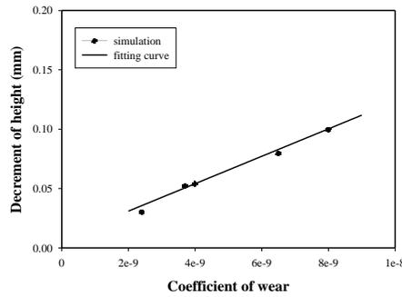
**Figure 4:** Decrement of height by wear coefficient of bearing at 10,000 revolutions
