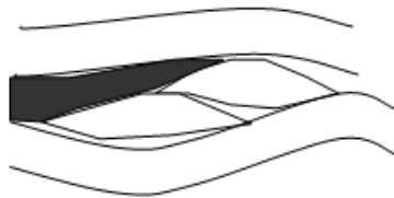
Figure 9. Two bundles aside defect
