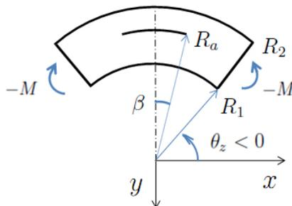
**Figure 1:** Schematic of the problem of a curved beam with a circumferential crack
