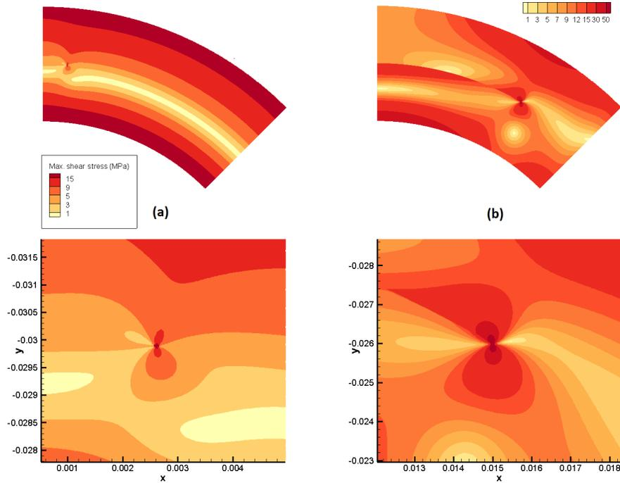
**Figure 6:** Contours of constant  $\tau_{max}$  with the corresponding zoomed view of the crack tip obtained by Tikhonov-regularized MMC method for (a)  $\beta = 5^\circ$  and (b)  $\beta = 30^\circ$ , for the *sample beam*.
