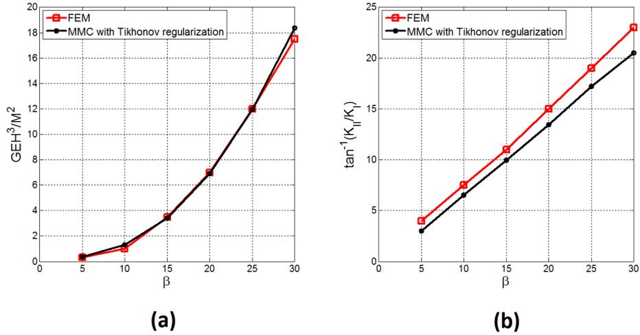
**Figure 5:** The results of Tikhonov-regularized MMC method (in black) and FEA with ABAQUS (in red, according to Lu et al. [1]) for (a) the nondimensionalized energy release rate and (b) mode mixity plotted against crack half arc angle,  $\beta$ , (in degrees) for the *sample beam*.
