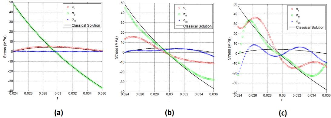
**Figure 4:** Instability of the solution *without* applying Tikhonov regularization method: The stress components on the moment-exerted boundary of the curved beam with  $R_1 = 24 \text{ mm}$ ,  $R_2 = 36 \text{ mm}$ ,  $R_a = 30 \text{ mm}$  and  $\beta = 5^\circ$ . Case (a): Total number of 14 stations,  $M = N = 3$ , Case (b): Total number of 24 stations,  $M = N = 5$ , Case (c): Total number of 33 stations,  $M = N = 8$ .
