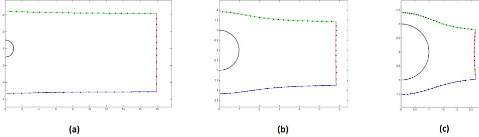
**Figure 3:** The mapped boundaries in the image plane for the beam with  $R_1 = 24 \text{ mm}$ ,  $R_2 = 36 \text{ mm}$  and  $R_a = 30 \text{ mm}$ . case **(a)**:  $\beta = 5^\circ$ , case **(b)**:  $\beta = 15^\circ$  and case **(c)**:  $\beta = 30^\circ$ . The unit circle (the mapped crack) is plotted in black. Due to symmetry only right half of the mapped region is presented.
