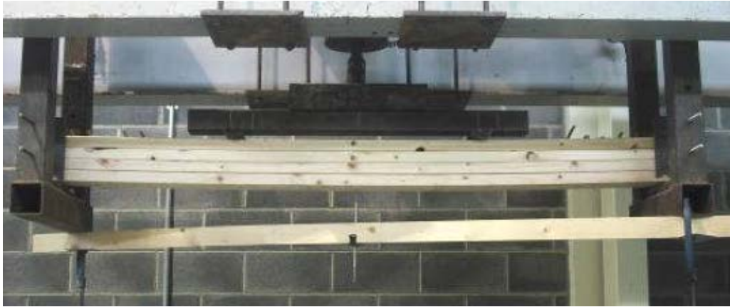
Fig. 2: Four-point bending tests: (a) test arrangement (in mm) (b) four-layer beam during test.
