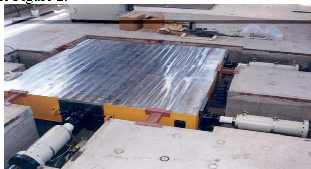
Figure 1: SST shaking table steel deck & horizontal actuators
