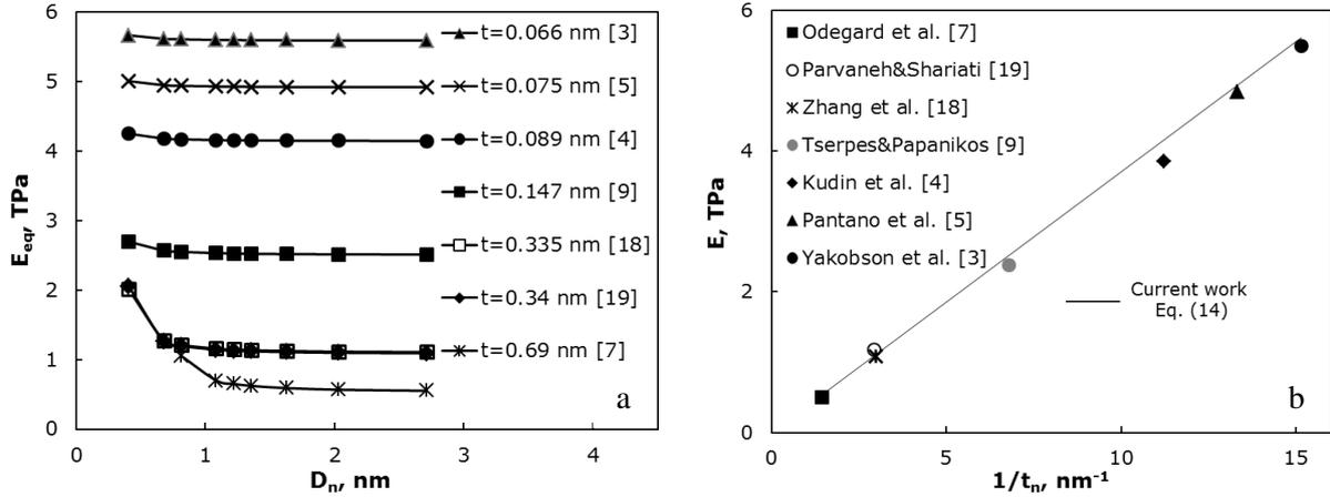
**Figure 5:** Comparative study: (a) evolution of SWCNTs Young's modulus with nanotube diameter for different wall thicknesses, (b) evolution of the Young's modulus of (10, 10) SWCNT with inverse wall thickness (values of  $D_n$  and fitting parameters from Tables 2 and 3, respectively)
