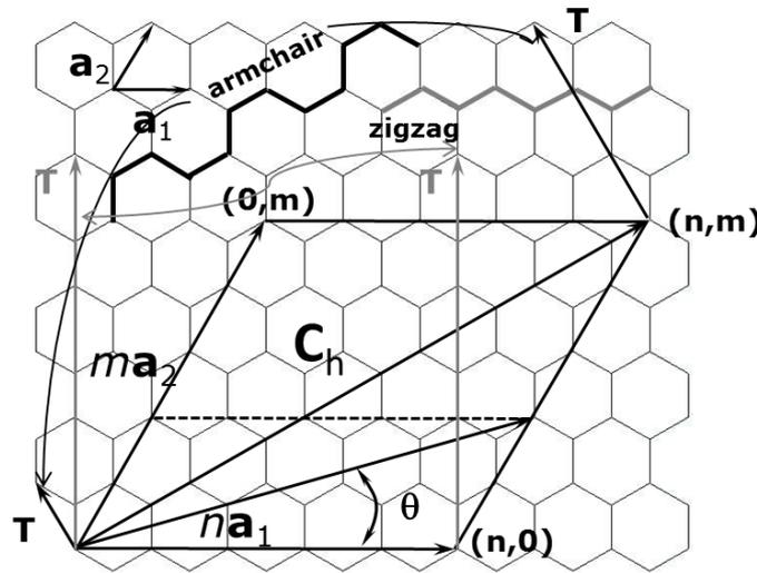
**Figure 1:** Schematic representation of the hexagonal lattice of the two-dimensional graphene sheet along with the definition of the chiral vector and description of SWCNTs formation
