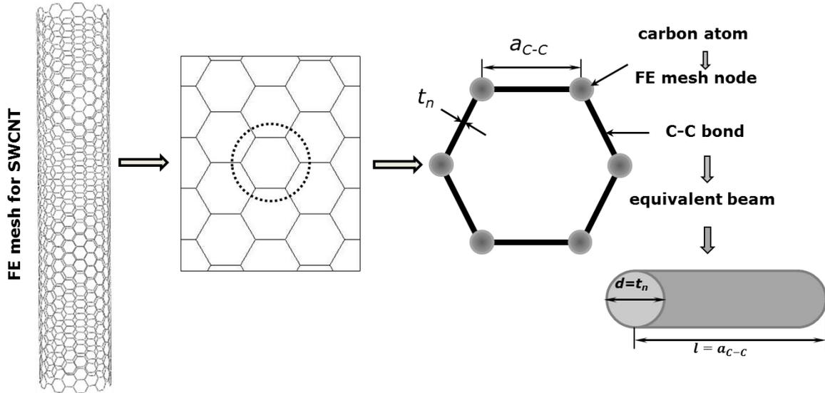
**Figure 2:** Modelling of SWCNT as a space-frame structure with beam elements substituting C-C bonds
