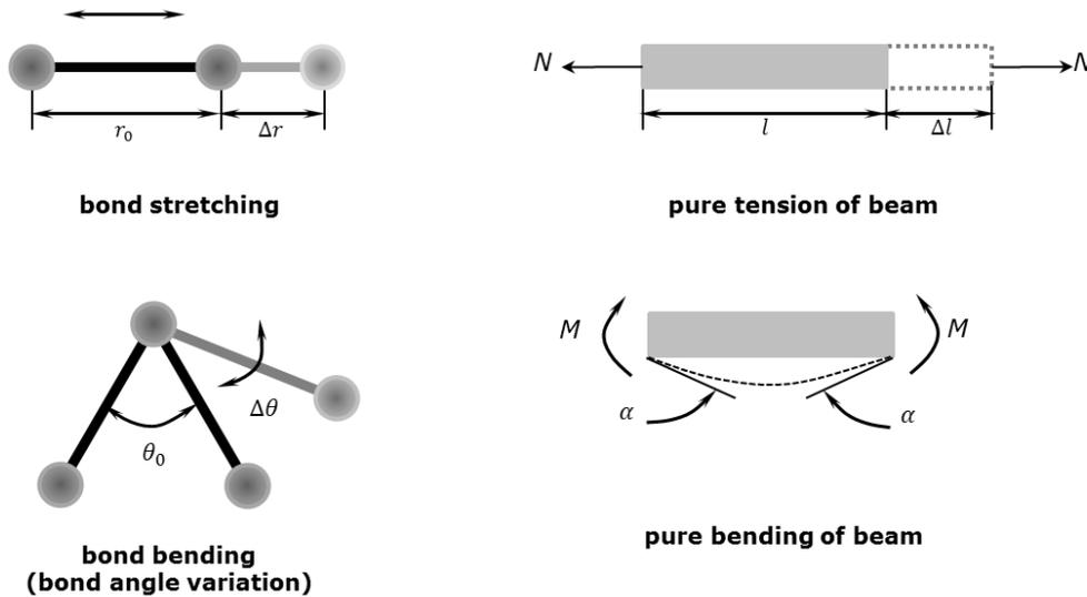
**Figure 3:** Equivalence between interatomic interactions in CNT and beam elements
