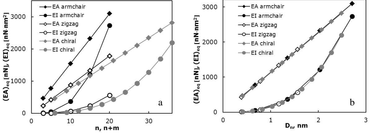
**Figure 4:** Evolution of the tensile,  $(EA)_{eq}$ , and bending,  $(EI)_{eq}$ , rigidities as a function of the chiral index,  $n$ , or  $(n+m)$  (a) and nanotube diameter,  $D_n$  for armchair, zigzag and chiral  $\theta = 19.1^\circ$  SWCNTs
