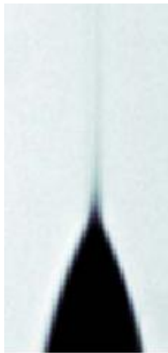
Figure 2: The formation of jet from an electrically charged viscous droplet. Top: numerical simulation from our model. Bottom: experiment from Grimm and Beauchamp.
