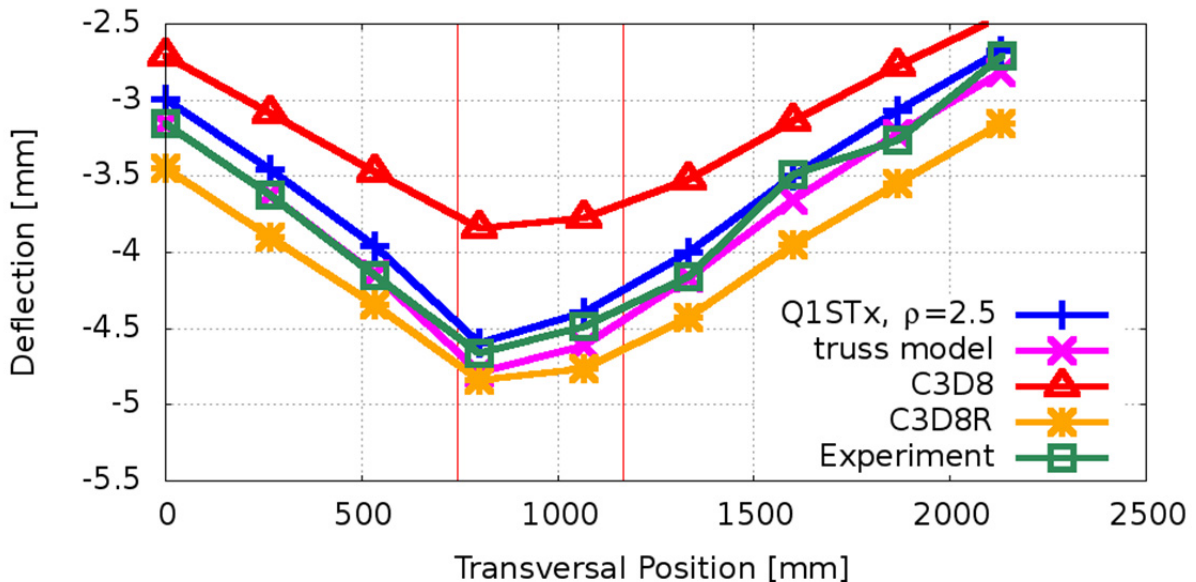
Figure 9: Deflection at the centerline, medium mesh. P=100 kN. The vertical red lines mark the area to which the load was applied.
