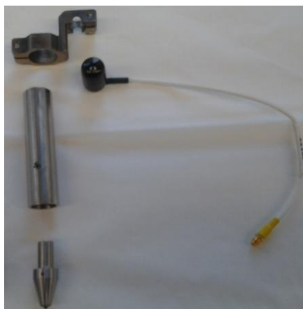
Figure 2: The capacitor sensor and the Vickers indenter
