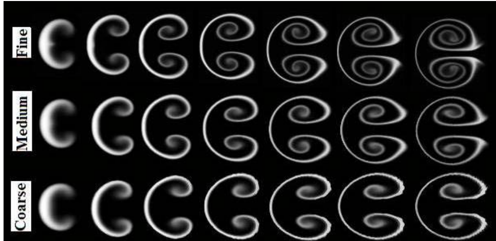
FIG. 2. Image sequence of SF 6 volume fraction at t=130, 220, 310, 400, 490, 560, and 650 \mu s after shock impingement on the coarse (left column), medium (middle column), and fine (right column) mesh resolutions. The shock has traversed the cylinder from top to bottom.
