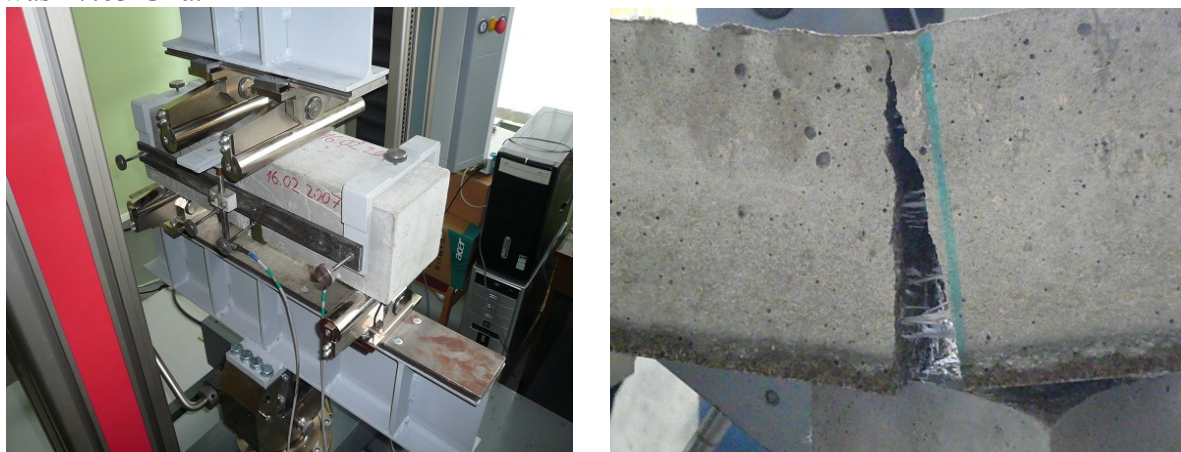
Figure 3: (a) Concrete prism, reinforced by four layers of glass fiber knitted fabrics, under four point bending; (b) Macro-crack opening with glass fiber yarns failure during prism bending under the increasing load.
