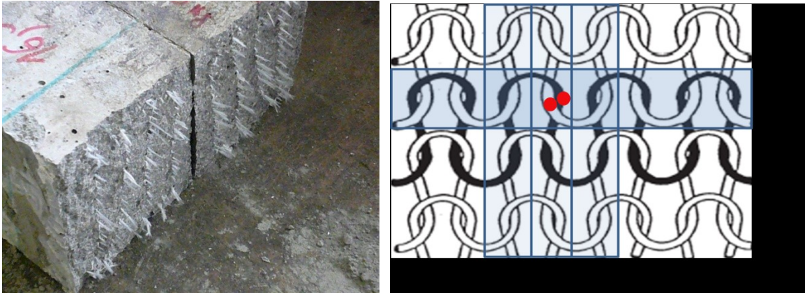
Figure 6. (a) Concrete prism, reinforced by four glass fiber knitted fabrics after failure; (b) Stretched yarns row in the macro-crack.
