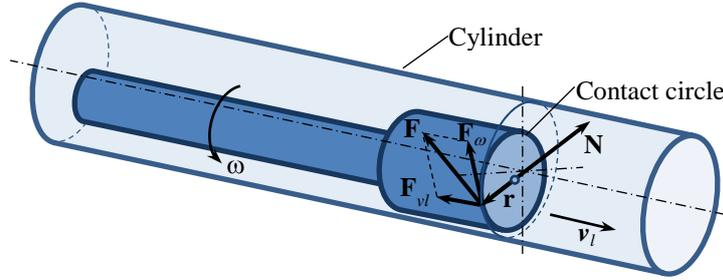
**Figure 2:** Circle-Cylinder contact model
