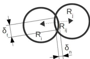
**Figure 1:** Description of the overlap between the particles
