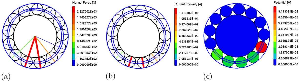
**Figure 9:** (a) Normal force (b) Electrical current and (c) Electrical potential, for  $F_r = 5820$  N with  $\epsilon = 0.3$
