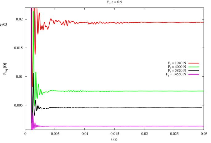
**Figure 8:** Electrical resistance versus time with different radial loads ( $\omega = 500$  rad/s and  $\epsilon = 0.5$ )
