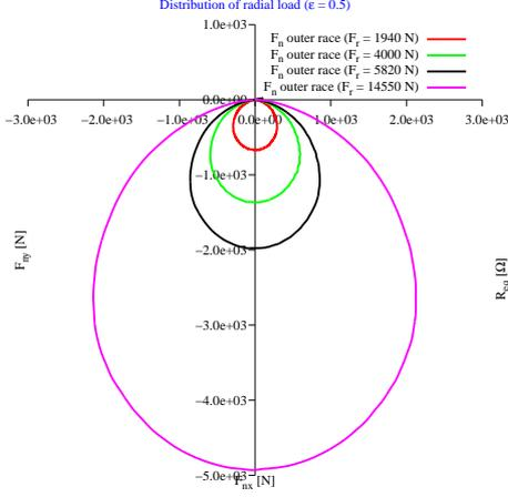
**Figure 7:** Radial load distribution of a ball on a rolling round ( $\omega = 500$  rad/s and  $\epsilon = 0.5$ )
