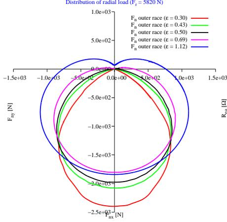
**Figure 10:** Radial load distribution of a ball on a rolling round
