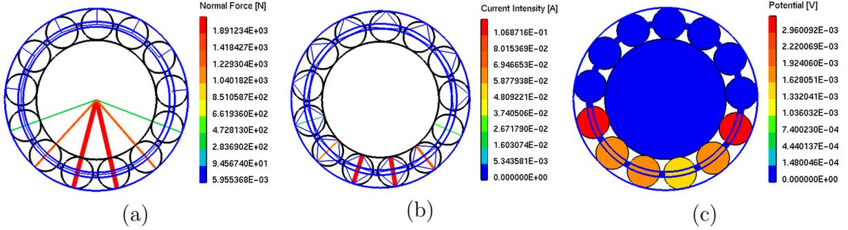
**Figure 6:** (a)Normal force (b)Electrical current and (c)Electrical potential, for  $F_r = 5820N$  with  $\epsilon = 0.5$
