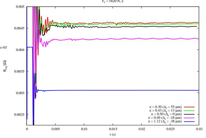
**Figure 11:** Electrical resistance versus time with different load parameters ( $\omega = 500$  rad/s and  $F_r = 5820$  N)
