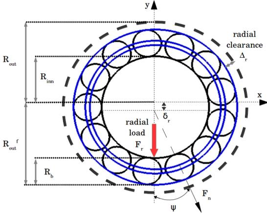
**Figure 3:** Characteristic dimensions of the ball bearing
