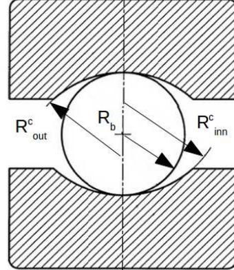
**Figure 4:** Compliance of the bearing rings
