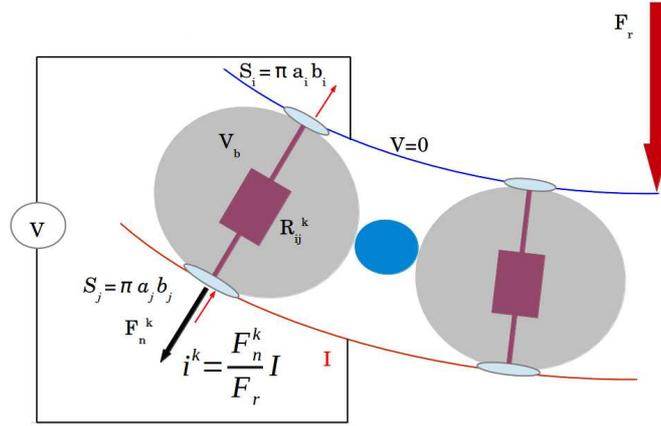
**Figure 5:** Illustration of electrical transfer in a rolling element
