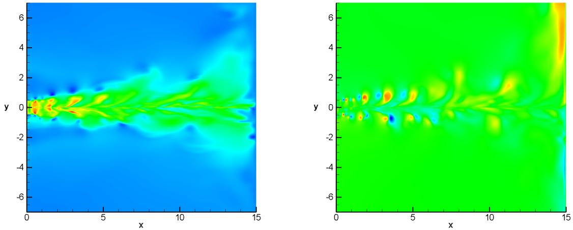
(a) axial velocity field in a 2D section.
