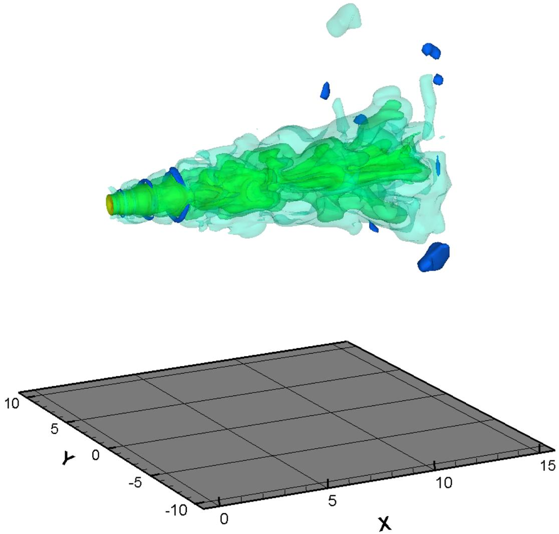
Figure 4: Three-dimensional view showing the axial velocity field as a whole.
