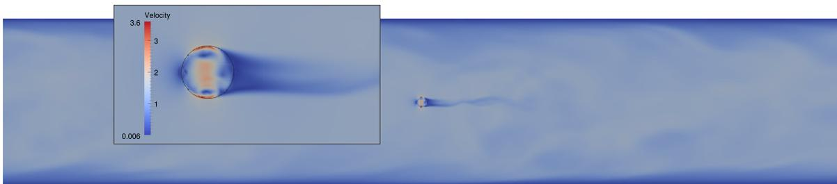
**Figure 4:** Velocity magnitude of the flow around the bubble in the turbulent pipe flow at  $t^* = 40$ .
