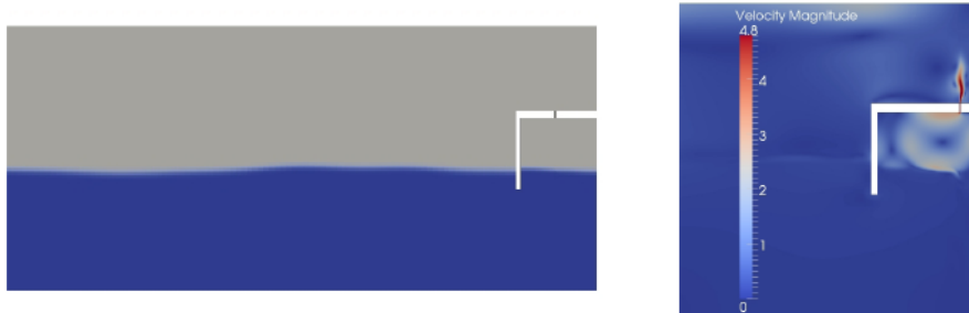
Figure 1: (left) Snapshot of the domain used for the simulations. (right) High velocity of the air through the orifice.
