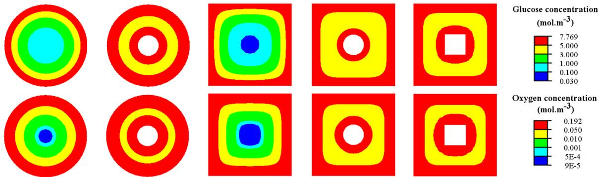
**Figure 3:** Glucose and oxygen steady-state radial distributions for the five different geometries. Profiles obtained at  $z=2.5$  mm.
