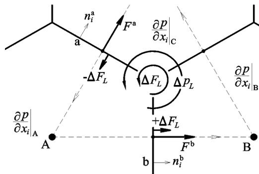
Figure 1: FLOP method variables assembly
