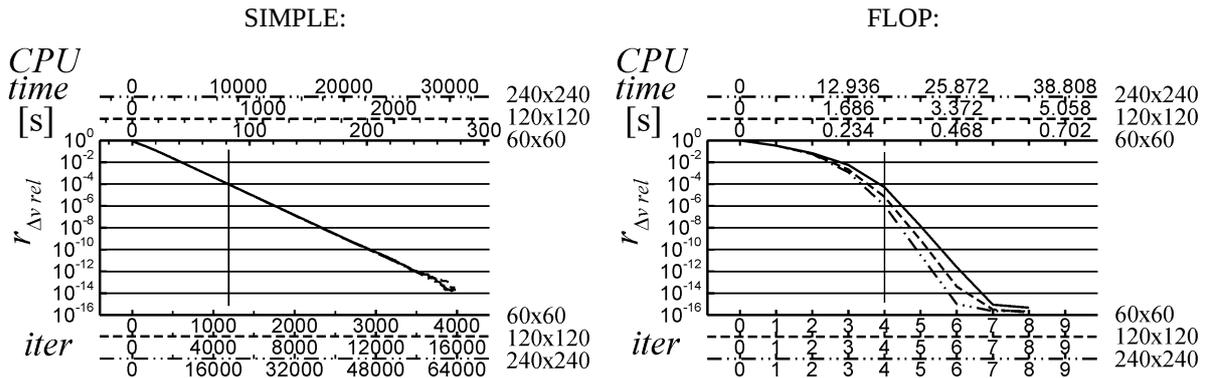
**Figure 3:** The convergence histories of the solution procedures for 2D lid-driven cavity laminar flow at  $Re = 100$ , solved for three different mesh sizes. The convergence histories are given in terms of the average relative difference in velocity field in respect to the own solution obtained at machine precision -  $r_{\Delta v, rel}$ .
