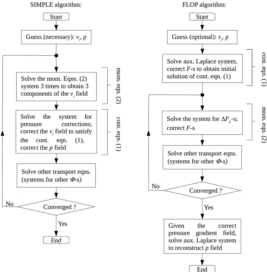
Figure 2: SIMPLE and FLOP algorithms procedures
