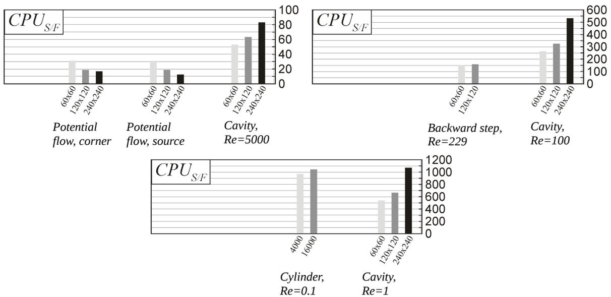
**Figure 4:** Efficiency comparisons of SIMPLE and FLOP algorithms in terms of CPU time ratios (SIMPLE/FLOP).
