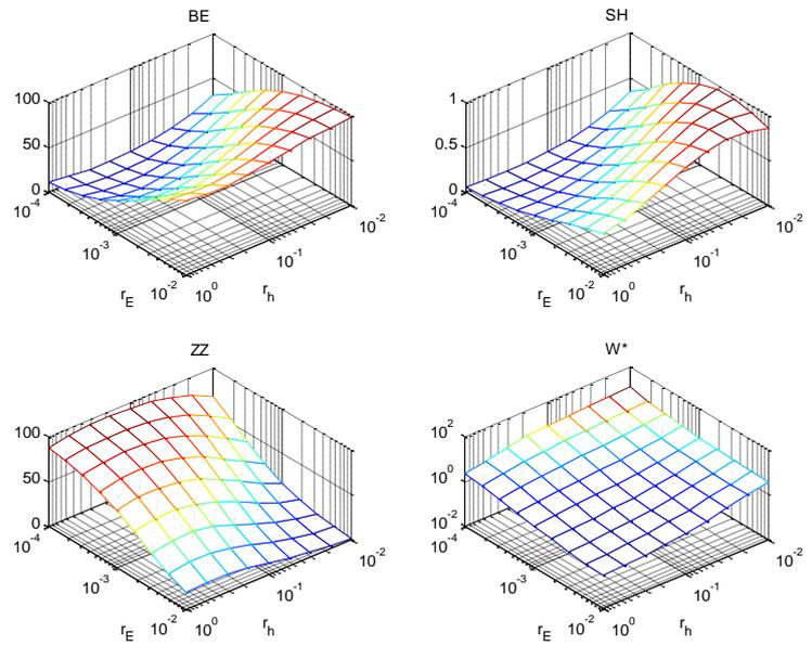
**Figure2:** Problem 3PB, sandwich-like stacking sequence. Bending, shear, and zigzag contribution to the maximum deflection and non-dimensional maximum deflection for  $\lambda=26$ .
