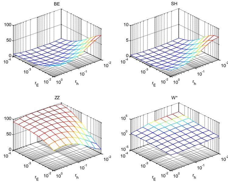
**Figure1:** Problem 3PB, sandwich-like stacking sequence. Bending, shear, and zigzag contribution to the maximum deflection and non-dimensional maximum deflection for  $\lambda=8$ .
