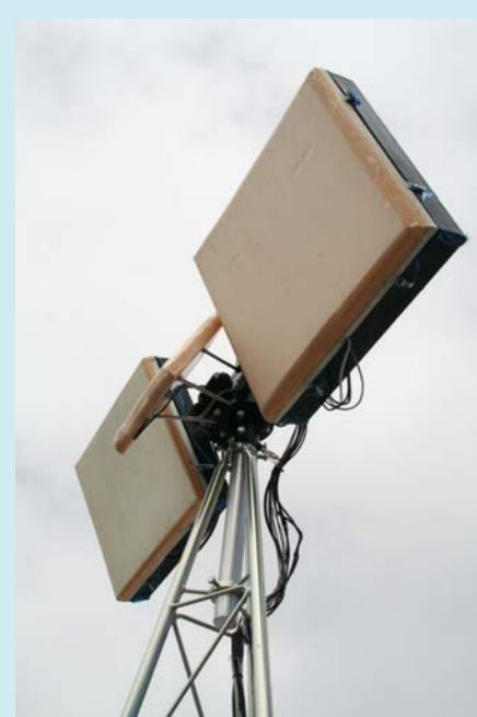
griPAU instrument: down-looking antennas for GNSS-R and L-band radiometer, up-looking antenna for GPS-receiver
