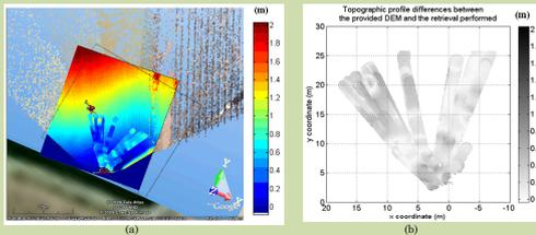
Figure 3. Topography retrieval performed over a barley field at REMEDHUS (Zamora) SMOS CALVALA SITE, 2009. (a) Topography retrieval performed by the SMIGOL-Reflectometer superimposed to the field DEM and (b) difference between the DEM and the retrieved topographical profile map.
