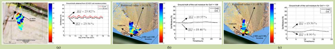
Figure 5. Soil moisture retrieval achieved by processing the SMIGOL-Reflectometer measurements (left) and ground truth values (right) for (a) a wheat field (Palau d'Anglesola, Lleida, 2008), (b) a barley field (Vadillo de la Gueña, Zamora, 2009) and (c) a barley field (Palau d'Anglesola, Lleida, 2010)
