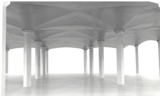
Figure 1: Design of a vaulted floor system without ties underneath the vault.
