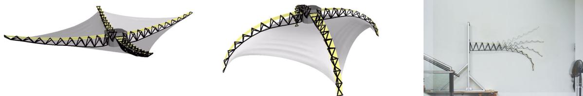
Figure 1. (Left) and (Middle) Dry and wet state of multi-truss assembly. (Right) 2 meter truss test
