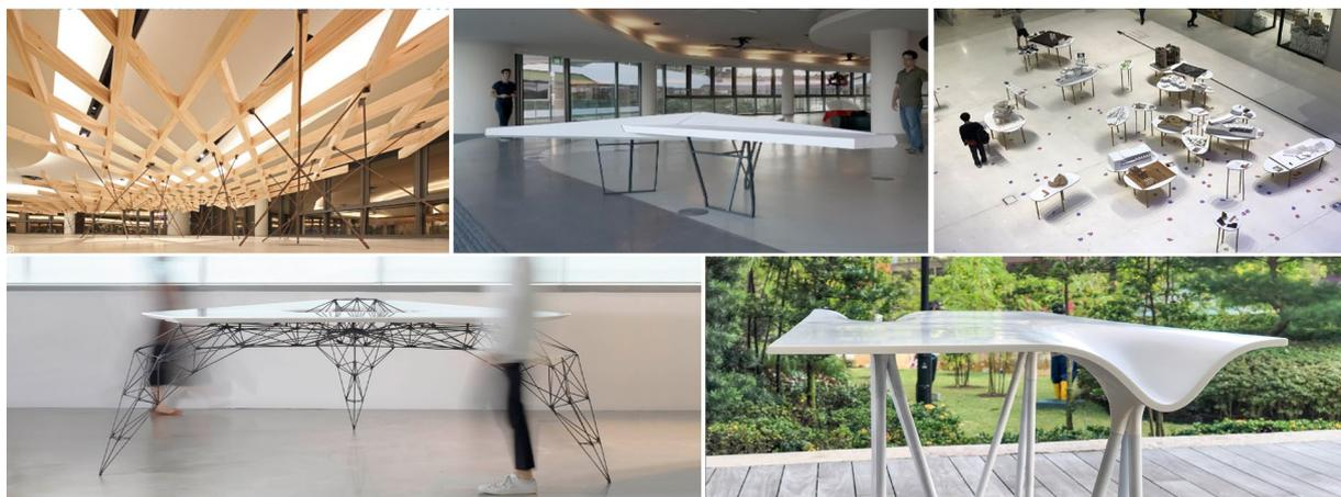
Fig 1: a) Timber modular grid system on rebars; b) Cardboard structural reciprocal table with CNC Zund cutter; c) Parametric tables using bamboo legs with bespoke PLA 3D printing; d) Space frame table using metal 3D printing; e) OH Platform for the Venice Biennale, using thermo-form table tops and nylon 3D printing joints.
