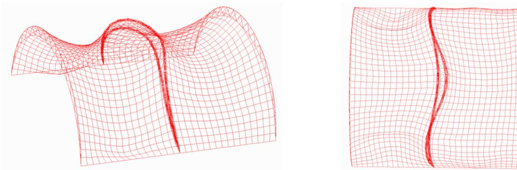
In the equilibrium state of the structure the classical eigenvalue problem is solved [2] to obtain the critical multiplier of the actual load. The elastic and the geometric stiffness of the membrane and the truss elements, respectively, must be selected to safely withstand the destabilizing effects.
