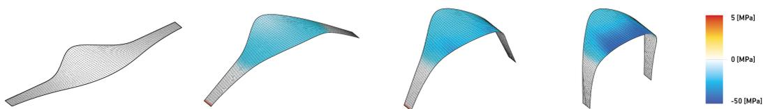
**Figure 1:** Process of forming a flat sheet (left) into a predefined form (right) showing stress in the bottom fibre
