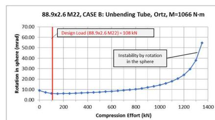
It is concluded that in all cases the instability of the node appears once design loads are largely exceeded, so the linear superposition of axial and flexion for checking a bolt's section can be admitted.
