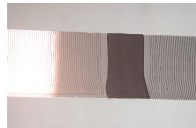
Test of a seam, sliding of yarns
