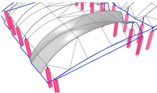
Figure 5: Typical module A with intermediate central cable
