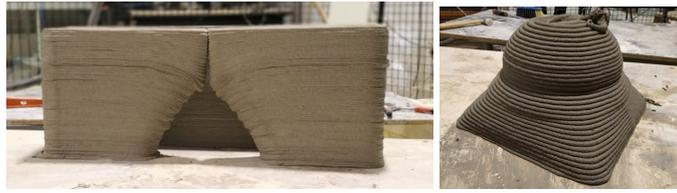
**Figure 2:** 3d printed arch using variable layer orientation (*left*) and dome on squinches (*right*)
