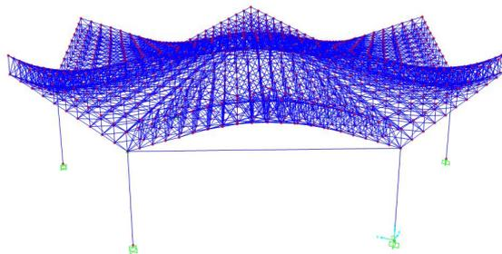
Figure(1) long-span prestressed double-layer composite torsional reticulated shell
