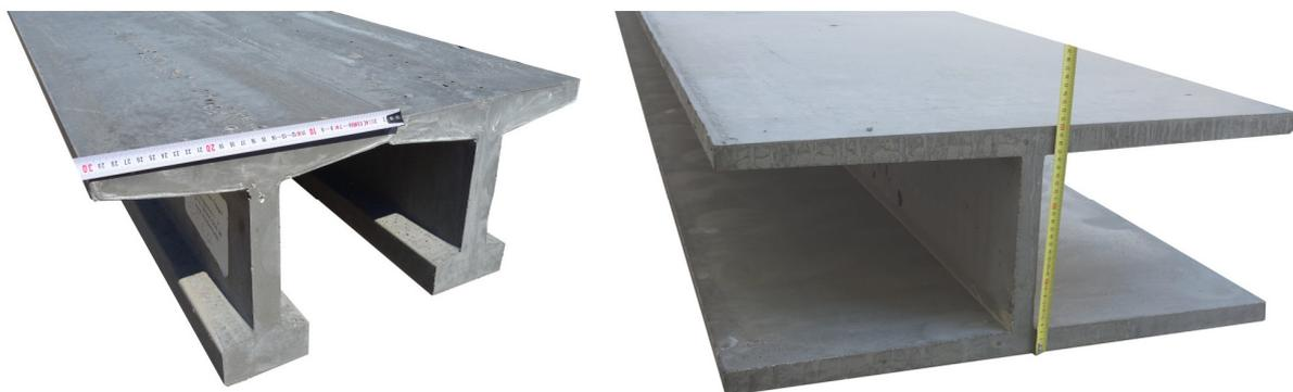
Figure 1: CFRP reinforced T-beam (left) and slab-element (right)
