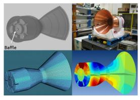
The experiments enabled the validation of the numerical model and made the determination of the acoustic damping by baffles with different number of radial blades possible.
