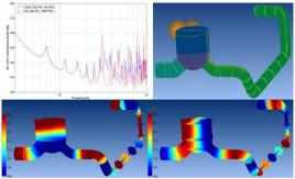
pressure drop due to the turbines. At the end the gas generator combustion chamber acoustics could reliably be characterized under consideration of hot gas parameter, flow and boundary condition as given.
