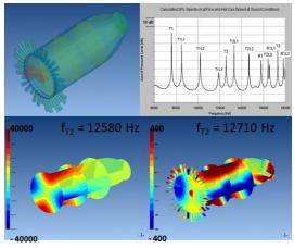
pressure spectrum of the untreated combustion chamber is given. The estimation of necessary amount of cavities has been done using available in-house codes based on MATLAB. The numerical model shows a drastic reduction of the modal sound pressure levels inside the combustion chamber if tuned cavities were included.
