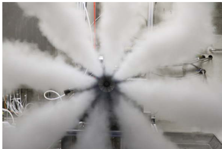
Figure 2: Test with HTP catalyst chamber carried on 17.12.2012
