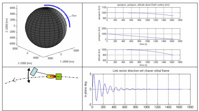
The perigee is lowered to 50km with a continuous 30mn long braking. The debris is pulled by a 100 meters long wire and oscillates behind the chaser. This preliminary simulation includes a full 6 dof dynamics of the chaser.
