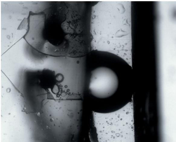
Figure 2: Electrolytic decomposition of concentrated HAN solution in the micro-combustion chamber.
