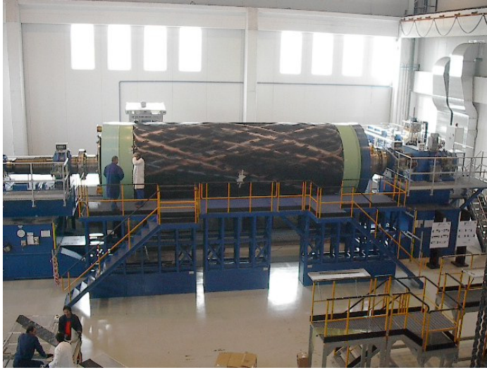
Fig. 1 P80 SRM filament winding phase
