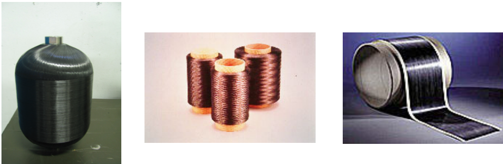
Fig. 2 Standard Small Vessel specimen with HXE-23 prepreg and raw materials carbon-epoxy prepreg TOW and TAPE
