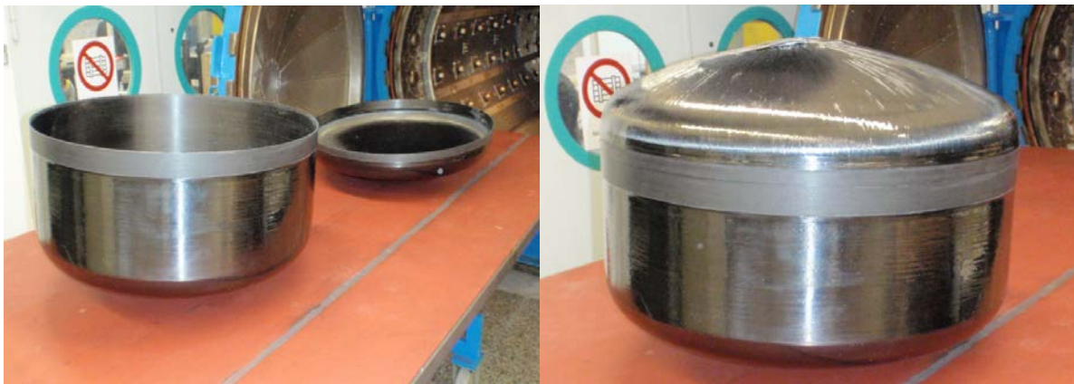
Figure 2: Tank with bandage in test production run at DLR [2]
