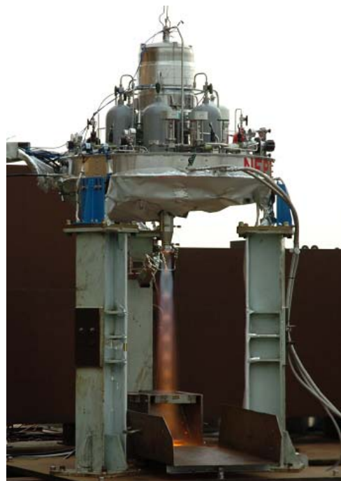
Figure 1. Appearance of propulsion system BBM equipped with \text{N}_2\text{O} /ethanol engine burning.
