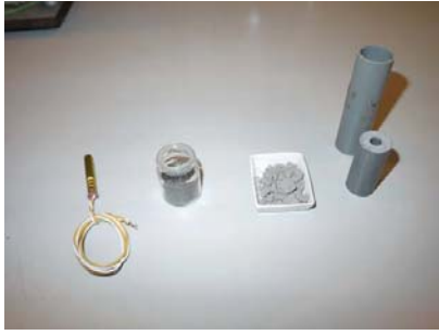
Figure 2: Pyrotechnic cartridge components
