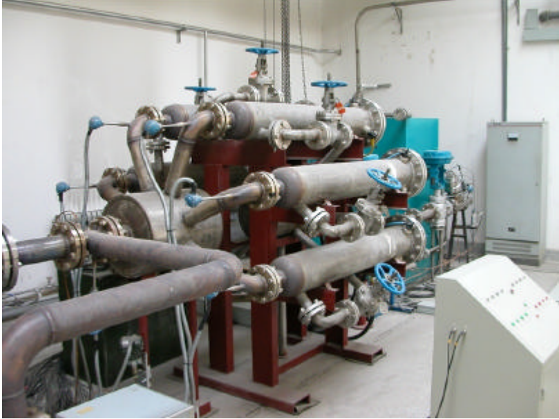
Fig.1 direct-connect resistance heated facility
