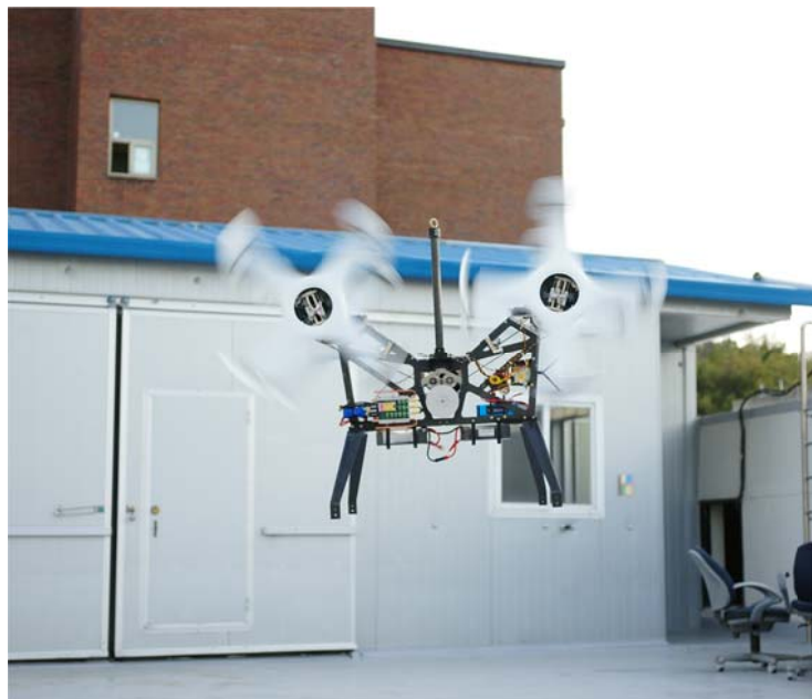
Fig. 2 Hovering test of MAV cyclocopter
