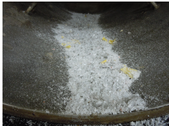
Fig. 2. Fragmented fuel after blasting (PMMA)
