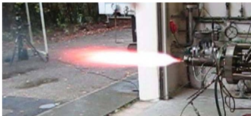
Fig. 3: Test run of a gel model rocket combustor at M11 test complex at DLR at Lampoldshausen test site
